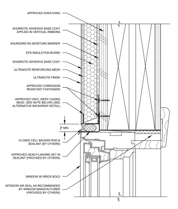
NOTE: MAINTAIN <sup>1</sup>/<sub>8</sub> SPACE BETWEEN BEVELED INSULATION AND WEEP CASING BEAD.
